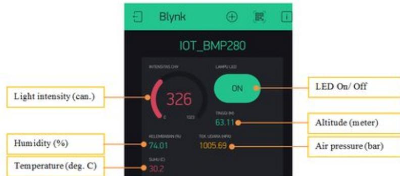
Figure 4. The dashboard in the smartphone using Blynk app for parameter monitoring
